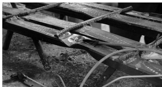
**Figure 7.** *Local buckling in the top angles at collapse*
