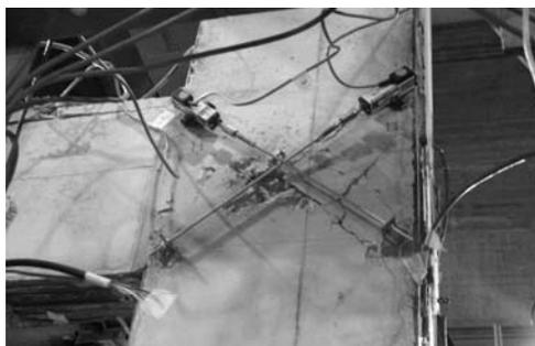
**Figure 13.** *Damage in the joint under reverse loading*
