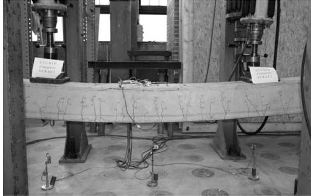
**Figure 9.** *Beam type B under four-point load bending*
